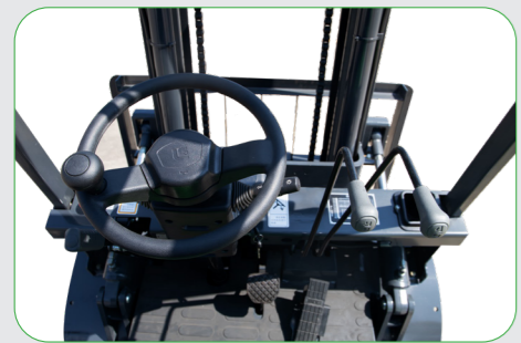
Ergonomic Cab • Ergonomically optimize the cab, reasonably layout the operating levers, and arrange the height of accelerator and brake pedal on the same plane, so as to effectively alleviate the driver's fatigue; • Equipped with a small steering wheel to increase the operating space
