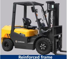
Integral stamping frame tail, structure is strong guirements of different attachment.
